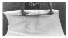
Fold the sail at the second or third batten and roll down to the boom. Never roll the sail around the boom, (boom fittings mark or damage the sail).
