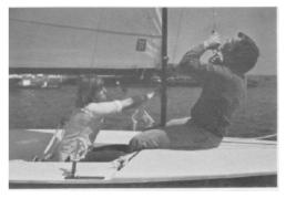
**57.** In order to put the ball into the halyard lock, use the rotation lever to turn the mast at right angles to the person on deck. At this point the halyard lock will be directly over head. (Remember this also for lowering the sail — use the lever to make the halyard lock accessible and then re-align the mast with the sail so that it will come down smoothly.)
