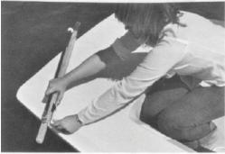
**59.** Install the tiller, pull hard on the downhaul line (if the water is deep enough) and cleat. Use as much tension as you can so that the rudder is always maintained in the straight down position. If it swings up, steering will become more difficult; if it swings all the way back, almost impossible.
