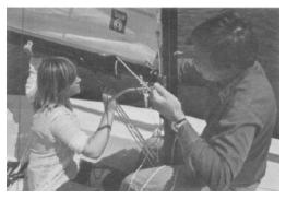
**58.** A hint for windy days. Pull the outhaul very tight to make sure the sail is completely flat. This greatly reduces the tendency of the boom to flog from side to side.
