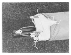
For storage other than overnight, release batten tension by springing the batten ties out of their notches. It is not necessary to untie them. Tension the ties by springing them back into their notches before next hoisting the sail (fig. 34).
