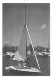
**56.** When the sail is almost all the way hoisted, the person in the cockpit should assist by raising the entire boom to take its weight off the sail.
