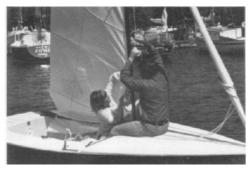
**55.** The procedure for hoisting the mainsail is the same as on shore, however, one person sits on the deck with a leg on either side of the mast; the other person sits on the centreboard capping or thwart. The person on deck should hoist and the other guide the sail into the groove. In particularly windy conditions, the boat will be more stable at the dock with the heavier person in the cockpit, and not as shown in the picture!
