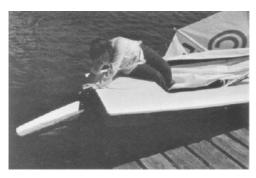
**53.** Make sure you push the rudder all the way down until the spring clip locks under the top gudgeon. Note that the blade is in the up position requiring no depth of water. Do not install the tiller yet as it will only tend to catch the sail while hoisting.
