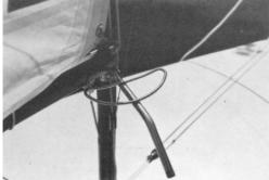
**48. When sailing on any other course** (ie reaching or running), lower the lever slightly and rotate it even further. Then raise it and lock it behind the plastic stop as shown in these two photographs taken from opposite sides of the sail. This is important as the mast will usually flip out of rotation (only annoying, rather than anything else!) as soon as the mainsheet is eased for reaching.
