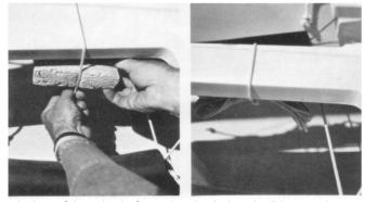
**43.** A useful method of carrying the halyard tail is to make a loop of shockcord around the centerboard capping. Use this to carry a sponge for cleaning up the boat and carry your halyard tail under the capping between sponge and shockcord.
