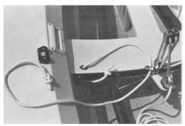
**31.** Install a traveler control line on each side of the thwart as shown. A figure-eight knot tied to the short end will stop the line from slipping through the eye.
