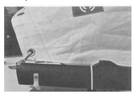
**37.** Attach the tack of the sail to the boom at the forward end with a shackle.
