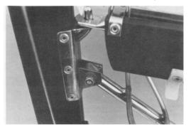
**45.** Before going on the water, familiarize yourself with the operation of the mast rotation lever. The locknut holding it to the mast should be adjusted so that the lever can readily be moved up and down but still stay in place when placed in the normal up position as shown above in fig. 44.
