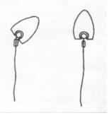
It also helps if the mast is aligned exactly in the direction of the sail so that the batten protectors do not bind on the back of the mast. Make sure the boom vang is slack and not cleated.
