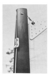
**41.** Hoist the sail until you can engage the small ball on the wire under the jaws of the hook (halyard lock). When this is done you can release the tension on the halyard and it will stay up under all conditions until you pull it down and out to release it. Push the boom back down on the gooseneck pin until it clips under the lock.
