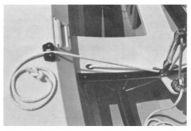
The traveler lines are cleated using the cam cleats mounted on the side decks.
