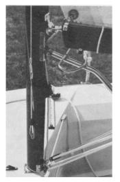
**42.** When the halyard is locked at the top of the mast, pass the loop of the shockcord under the small black hook and remove the rope tail completely.
