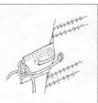
**34.** To secure and tension the batten at the leech, start from one eyelet, pass the batten tie through the hole in the batten, through the other eyelet, then knot both ends of the tie across the notch in the end of the batten. Tension the tie until the sailcloth along the batten pocket just shows tension.
