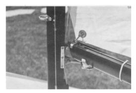
**46. When sailing close hauled**, the lever will be rotated either to the left or right until the "ears" come up against the plastic stop on the boom. When you are sailing on port tack the lever is rotated to starboard as shown in the photograph.
