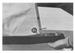
**36.** Attach the outhaul of the mainsail to the shackle at the end of the boom. Make sure the wires are all running smoothly and are not kinked.
