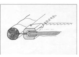
**33.** Install the battens in the sail. Each batten has two end caps. The end cap with a small hole and a V-notch belongs at the leech of the sail; the other end should be inserted into the pocket. Ensure that this end of the batten fits snugly into the plastic protector fitted on the sail at the forward end of the pocket.
