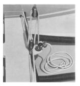
**30.** Rig the mainsheet as shown, starting from front to back through the double block hung from the boom.
