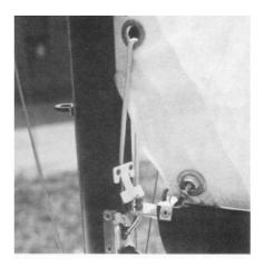
**44.** You will find the luff downhaul (cunningham) attached to the gooseneck fitting. Undo the end at the fitting, pass it through the grommet (about 6" up the luff) and then back down under the pin and knot it.
