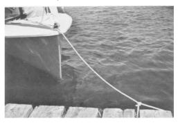
Check and tighten all inspection hatches. Tie a painter to the bow fitting which can be left in place while on the water.
