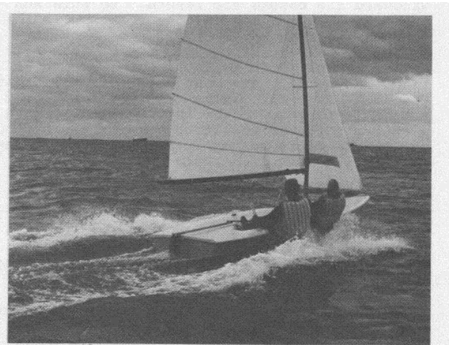
Fig 13 The Tasar sails fastest when it is guided smoothly like a high speed auto or aircraft, and any coarse or rapid tiller movements will slow the boat.
