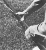
10. Assemble the mast by first sliding the top section into the lower section until the stainless steel metal tang is right against the lower section. Take both ends of the halyard (shackle and rope tail) and secure temporarily near the bot tom of the mast. This is done so that you don't put the mast up and find you have left the halyard shackle at the top!
