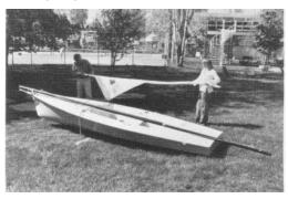
12. If the boat is sheltered from the wind it is not necessary to pre-roll the jib. If, however, you are trying to rig in a windy spot have your crew take the other end of the jib and roll it into a fairly tight roll. It will be much easier to raise the mast with the jib rolled than to have it flapping in the wind. See fig. 18 below.
