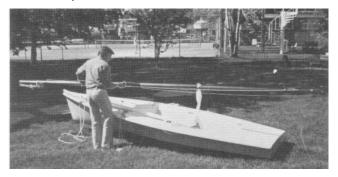
**17.** Lift the mast off the boat and place it vertically along side the boat. Do not place it on the ground if there is any
