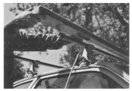
**4.** Most roof racks are not quite wide enough to properly transport a Tasar. This shows a rigging board with two wooden strips screwed onto the underside to position it over a roof rack. The padding has also been extended the full length of the board so that the boat can be put on from one side and slid across the rack. The boat is best supported on the flats of the side decks just behind the small bump where the foredeck meets the side deck.
