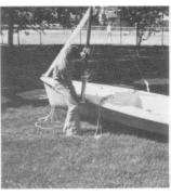
**18.** When the mast is steady and balanced, lower your grip and raise it straight up placing your strongest hand (right if right-handed!) under the base plug.
