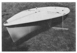
1. Place the hull, bow into wind, on its trailer, a soft surface, or a rigging board. We strongly recommend making a rigging board; it is simple and inexpensive and greatly simplifies rigging and working on the boat.
